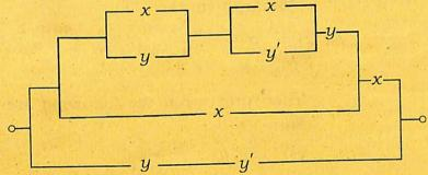
Draw an equivalent circuit as simple as possible. Show that current will flow through the circuit if and only if the switch x is on.
