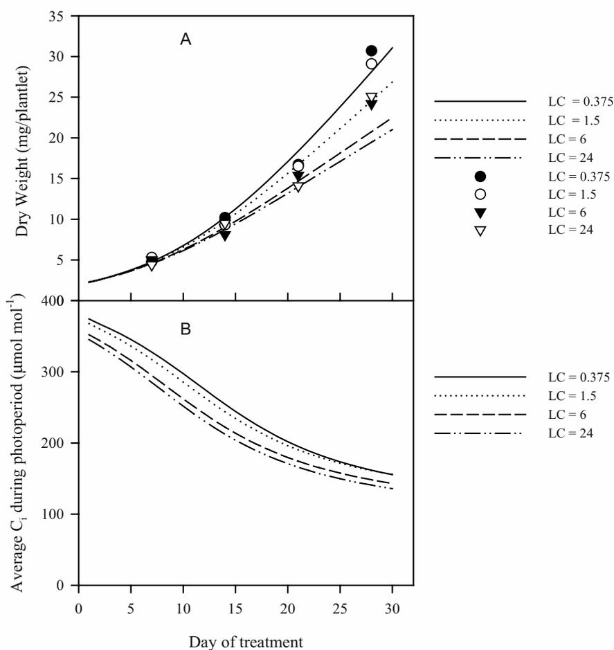
Figure 4. Simulated (lines) and weekly measured (symbols) dry weight of potato plantlets (A) and simulated average  $\text{CO}_2$  concentration in the vessel during photoperiod (B) under various lighting cycles over the course of the whole experimental period.
