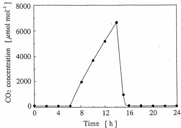
Figure 3. A diurnal change in CO<sub>2</sub> concentration in a culture vessel containing *Ficus lyrata* plantlets (Fujiwara et al., 1987). Dark period was from 6 to 14 h, and photoperiod was from 0 to 6 h and from 14 to 24 h. PPF at the culture level and air temperature in the culture room were  $65 \mu\text{mol m}^{-2} \text{s}^{-1}$  and 25 C, respectively.
