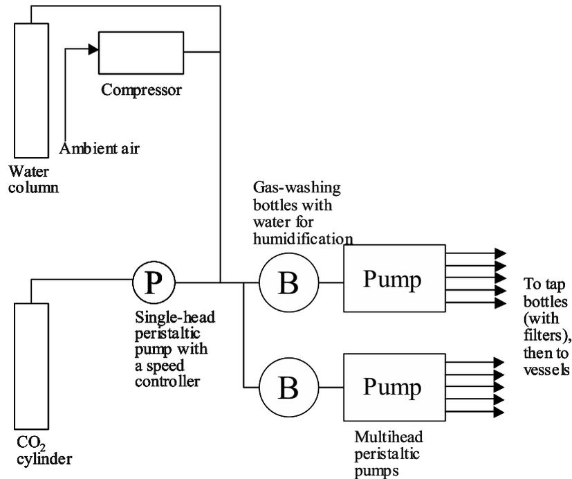
Figure 4. Basic components of the forced ventilation system developed by Erturk and Walker (2000a). CO<sub>2</sub> enriched air is pumped into each vessel (400 mL) through an air inlet and exited around the vessel lid.
