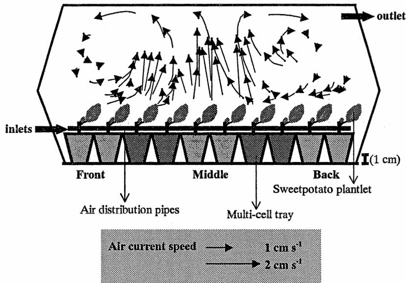
Figure 12. Two dimensional patterns of air currents in the culture vessel with forced ventilation using air distribution pipes on the plug tray with sweetpotato plantlets 6 days after transplanted (Heo, 1999). Vessel size: 368 mm long, 178 mm high and 170 mm wide, Air volume: 11.14 L. Forced ventilation rate:  $13 \text{ ml s}^{-1}$ . Number of air exchanges of the vessel:  $3.9 \text{ h}^{-1}$ . Air currents were observed as described in Figure 11.
