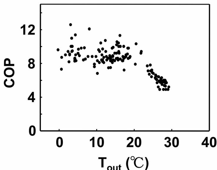
Figure 18. C.O.P. (Coefficient of performance of the closed system with a refrigerator) for cooling is as high as 8-10 when air temperatures inside and outside the closed system are 25 C and 0-20 C, respectively (Ohyama et al., 2002).
