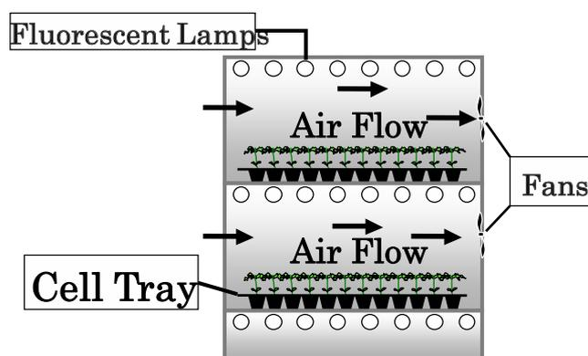
Figure 3. Cross section of multi-shelves (only two shelves are shown) showing the direction of air flow and positions of micro fans. This air flow guarantees the uniformity of microenvironments over the trays and within the transplant canopy.
