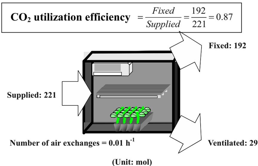
Figure 19. CO<sub>2</sub> utilization efficiency of the closed system, which is defined as the weight ratio of fixed CO<sub>2</sub> by plant photosynthesis to supplied CO<sub>2</sub> during the transplant production (Yoshinaga et al., 2000).
