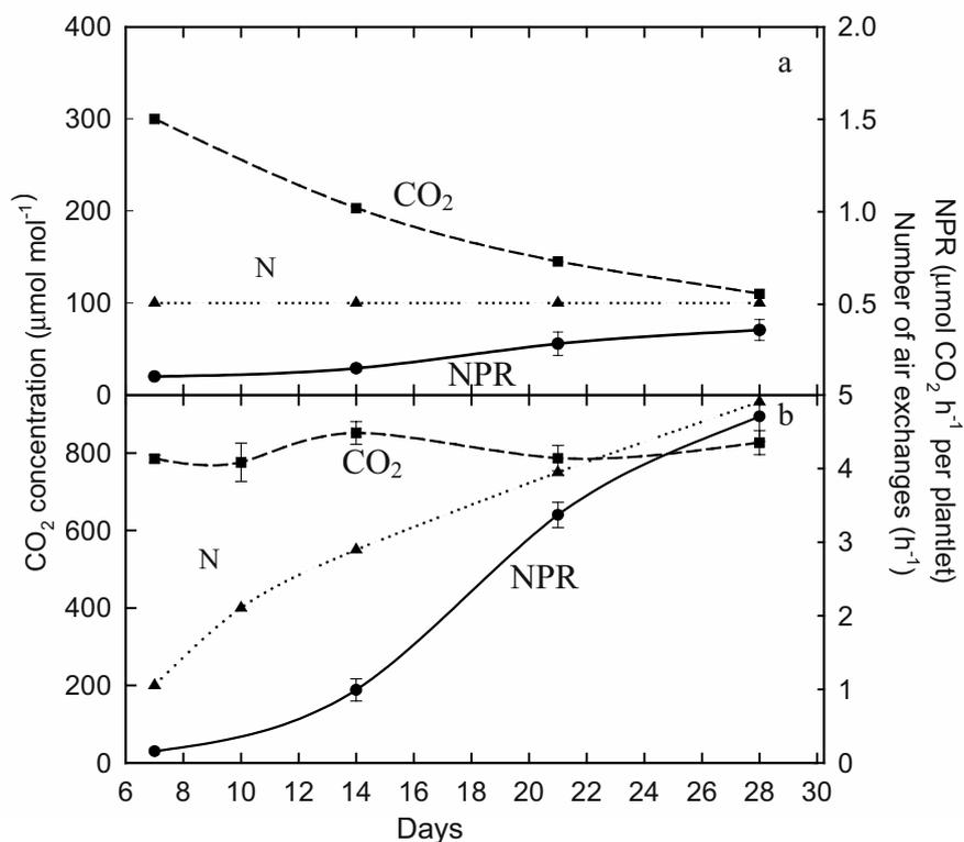
Figure 11. CO<sub>2</sub> concentrations (CO<sub>2</sub>), net photosynthetic rates (NPR) and numbers of air exchanges (N) of a culture vessel with *Eucalyptus* plantlets under (a) natural ventilation and (b) forced ventilation.
