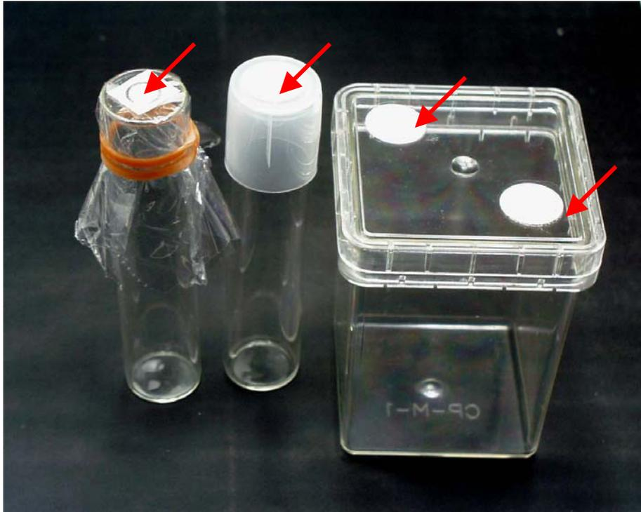
*Figure 3. Varieties of vessel lids with enhanced ventilation; arrows indicate the filters for ventilation.*
