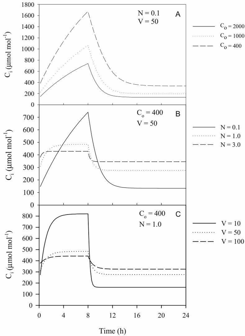
Figure 2. Simulated time courses of CO<sub>2</sub> concentration inside the vessel ( $C_i$ ) as affected by CO<sub>2</sub> concentration outside the vessel ( $C_o$ , Figure 2A), number of air exchanges ( $N$ , Figure 2B), and air volume per plantlet ( $V$ , Figure 2C). Dark period: 0 to 8 h; photoperiod: 8 to 24 h (Niu et al., 1996a).
