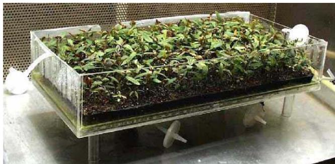
Figure 10. Scaled-up photoautotrophic culture vessel (picture taken after removal of the lid). The vessel was 610 mm long, 310 mm wide and 105 mm high (volume approx. 20 l) (Zobayed et al., 2000).
