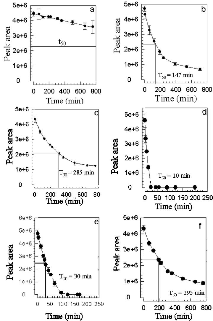
Figure 2.  $T_{50}$  measurements for the removal of injected ethylene from a 120 ml glass vessel capped in various ways. a) airtight system: sealed with silicone rubber bung; b) polypropylene disc; c) cotton bung; d) one adhesive microporous filter discs (filter pore diameter 0.45  $\mu\text{m}$ ; Millipore Corporation, USA) on the hole (8 mm) of the lid; e) Suncap closer (Sigma, USA) and f) aluminium foil functioning diffusively.
