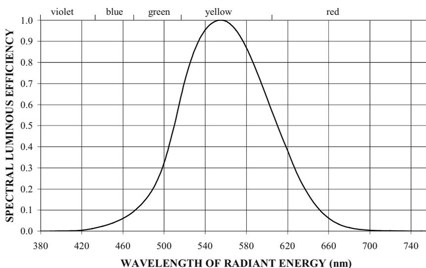
*Figure 2. Spectral luminous efficiency of humans. Human eyes are the most sensitive to the wavelength of 555 nm (yellow). Spectral sensitivity of a lux meter for measuring the illuminance is just the same as shown here. Thus, a lux meter is not suitable for measuring PPF and PAR.*
