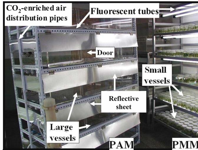
Figure 1. A culture module of the photoautotrophic micropropagation system using large culture vessels (PAM system) in the left and a culture module of the photomixotrophic micropropagation system using small vessels with natural ventilation (PMM system) in the right.
