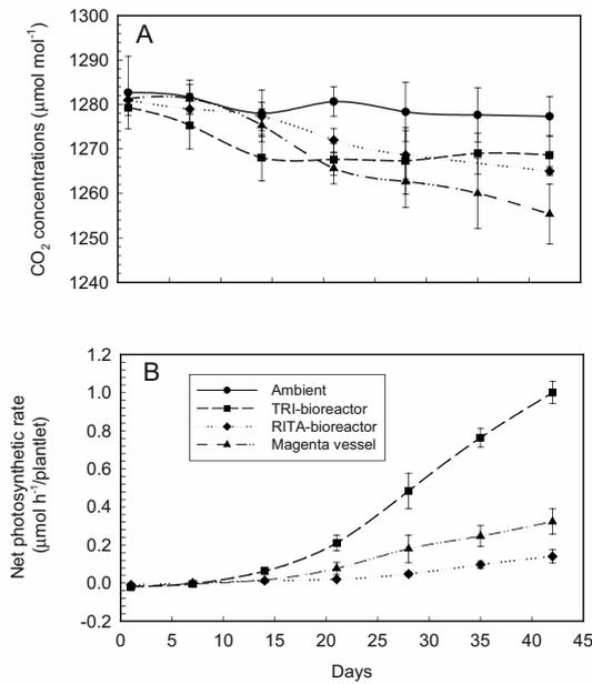
Figure 13. A, Carbon dioxide concentrations in the culture headspace of a TRI-bioreactor, Magenta vessel and modified RITA-bioreactor; B, net photosynthetic rates of coffee plantlets grown in a TRI-bioreactor, Magenta vessel and in a modified RITA-bioreactor (after Afreen et al., 2002b).
