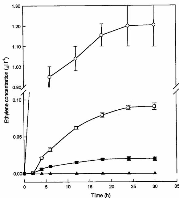
Figure 7. Time courses of  $C_2H_4$  concentrations in the vessels containing *Lagerstroemia speciosa* plantlets during the photoperiod, as affected by the number of air exchanges of the vessel (Zobayed, 2000). Vessels were capped with silicone rubber bung (open circle), cotton bung (open square), polypropylene film (solid square) and forced ventilation (solid triangle). The numbers of air exchanges of those vessels, respectively, 0.2, 1.1, 1.8 and  $6.0 \text{ h}^{-1}$ .
