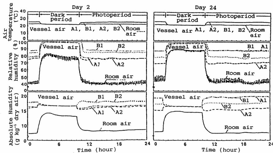
Figure 8. Daily changes of relative humidities, air temperatures and absolute humidities inside and outside the vessel with and without gas permeable film, and without and with *in vitro* potato plantlets 2 days and 24 days after transplanted in the vessel (Kozai et al., 1995b). A1: with filter and plantlets, A2: with filter and without plantlets, B1: without filter and with plantlets, B2: without filter and plantlets.
