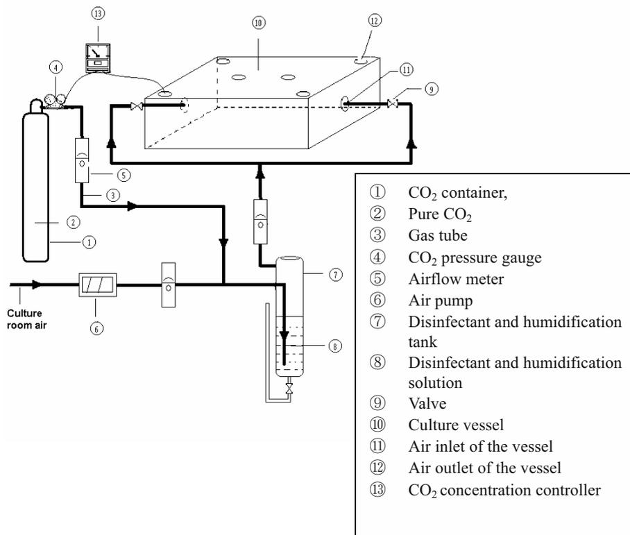
Figure 3. Schematic diagram of a forced ventilation unit for CO<sub>2</sub> enriched air supply.
