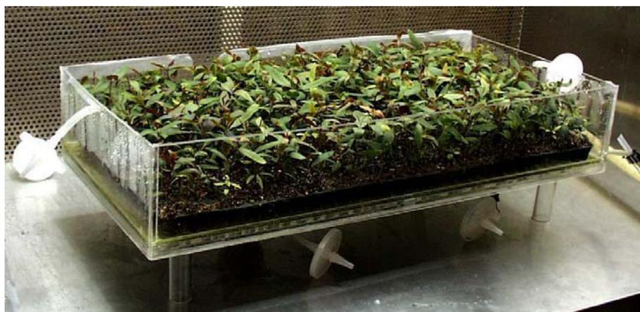
Figure 5. A large culture vessel (volume: 20 L) with a forced ventilation system developed by Zobayed et al. (2000). The vessel was 610 mm long, 310 mm wide and 105 mm high.
