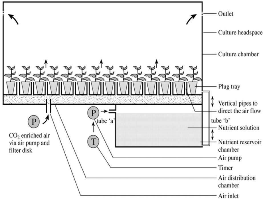
Figure 11. Schematic diagram of the Temporary root zone immersion bioreactor developed for growing cotyledonary stage somatic embryos under photoautotrophic conditions (after Afreen et al., 2002b).
