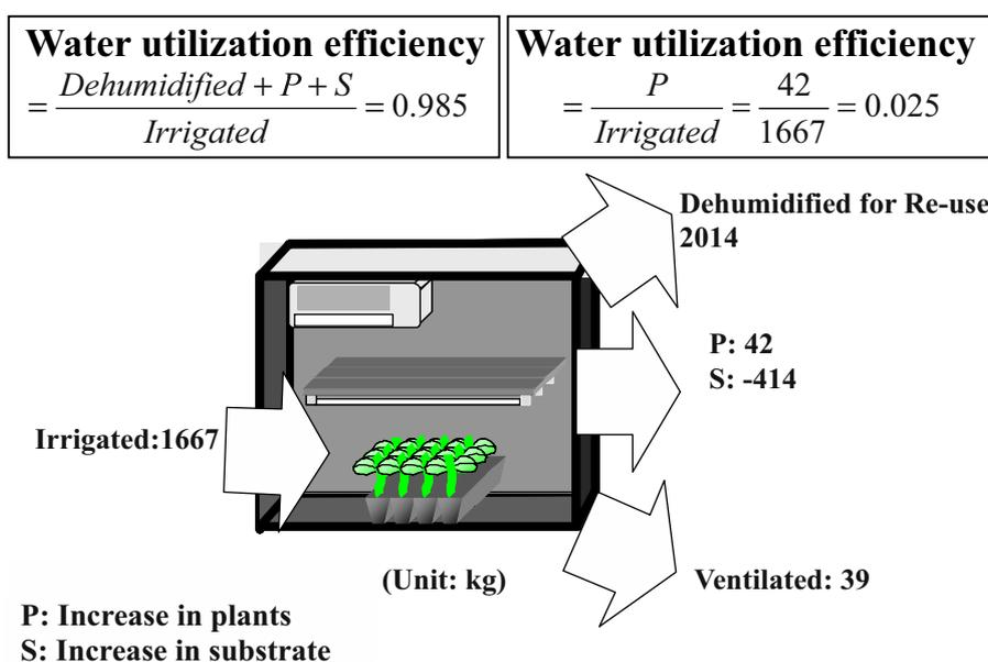
Figure 20. Water utilization efficiency of the closed system, which is defined as the weight ratio of water captured in plants or substrate to the supplied water during the transplant production (Ohyama et al., 2000b). Left: Water collected at the cooling panel (evaporator) is reused for irrigation. Right: Water collected at the cooling panel (evaporator) is not reused for irrigation.
