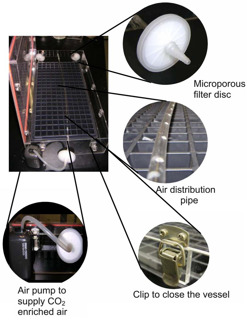
Figure 4. Different components of an ideal large vessel for photoautotrophic micropropagation (Zobayed et al., 2004).
