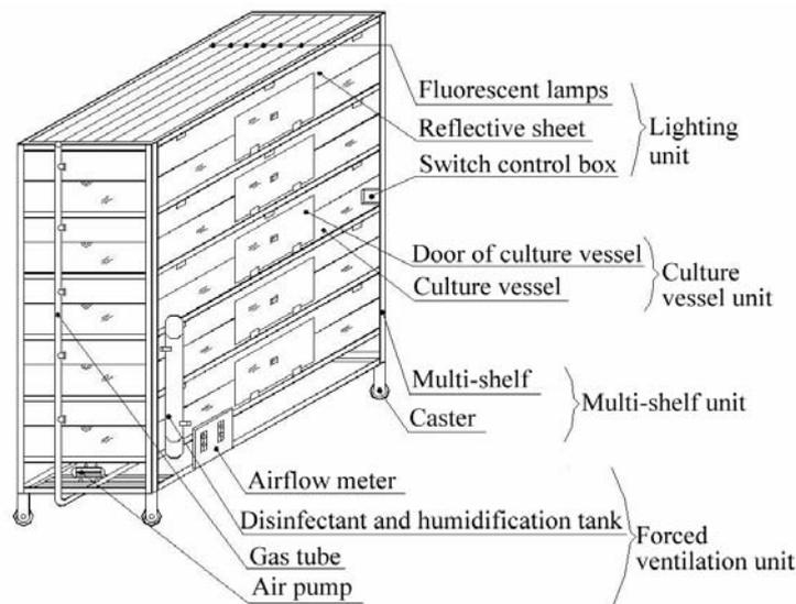
Figure 2. The culture module of photoautotrophic micropropagation system using large culture vessels with forced ventilation.
