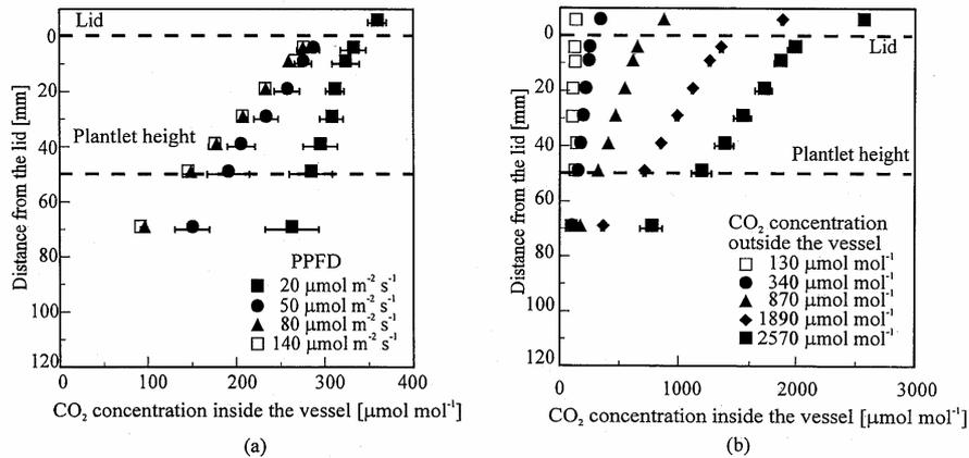
Figure 6. CO<sub>2</sub> concentration profiles in a test tube type vessel at (a) different PPFs and (b) different CO<sub>2</sub> concentrations outside the vessel (Ohyama and Kozai, 1997). The vessel contained a sweetpotato plantlet on sugar containing MS agar medium.
