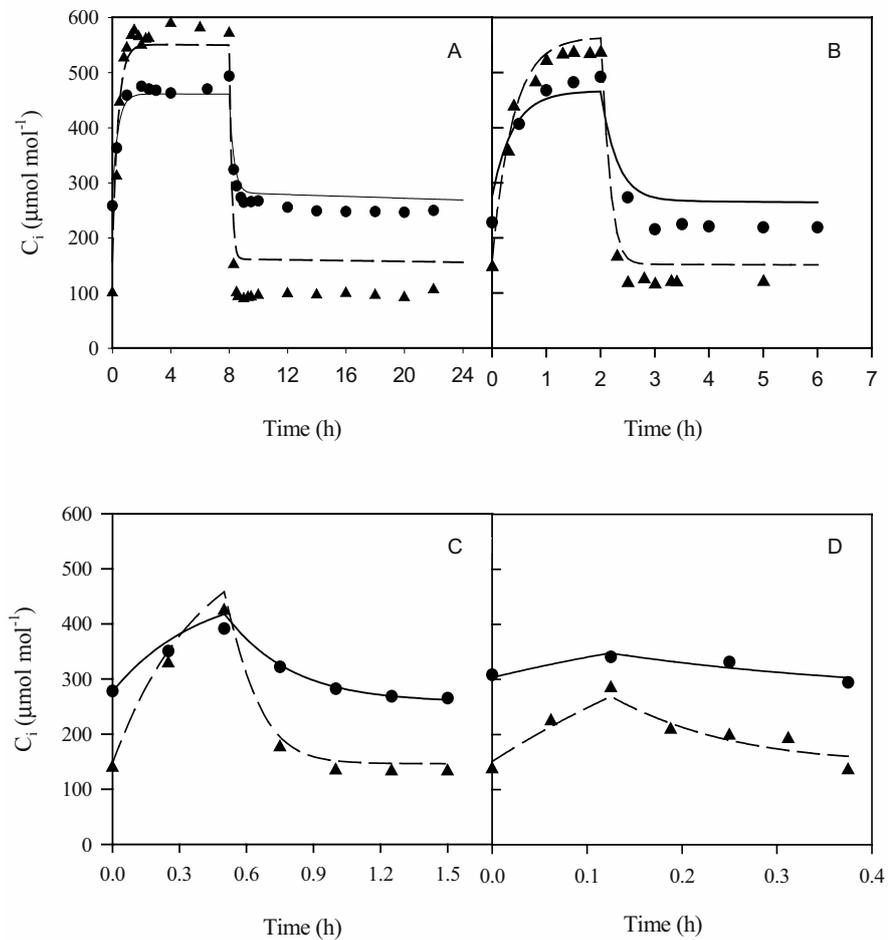
Figure 3. Simulated time courses of CO<sub>2</sub> concentration inside the vessel ( $C_i$ ) as affected by lighting cycles (24, 6, 1.5, and 0.375 h, with same ratio of photoperiod to dark period). Solid and dash lines represent simulated time course of  $C_i$  on days 7 and 21, respectively. Circle and triangle symbols represent measured  $C_i$  on days 7 and 21, respectively (Niu et al., 1997).
