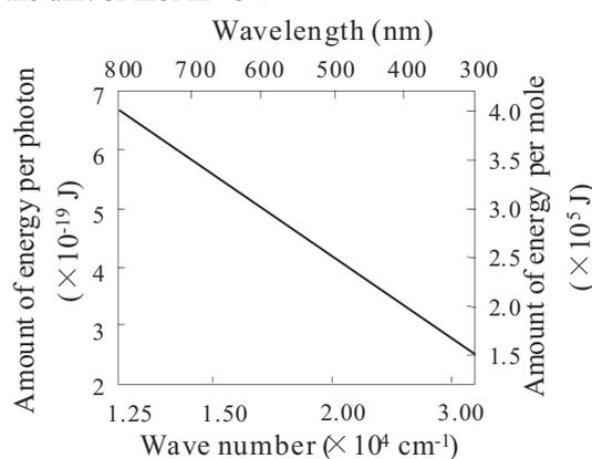
Figure 1. Amount of energy per photon and per mole as a function of wave number.
