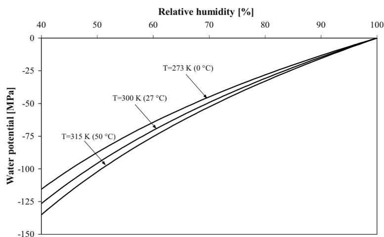
Figure 4. Water potential of air as a function of relative humidity at 273, 300 and 323 K. Water potential of air with 100% relative humidity is 0 Pa. Water potential decreases exponentially with decrease in relative humidity at a given air temperature.
