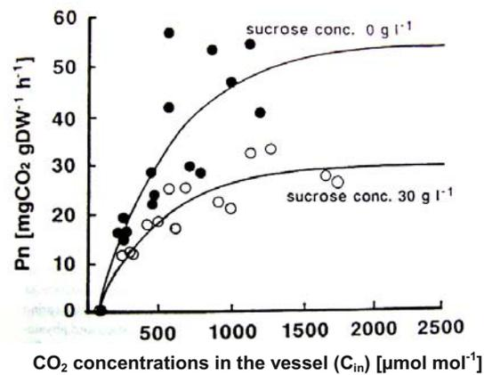
Figure 2. Net photosynthetic rates per leaf dry weight ( $P_n$ ) of potato explants as affected by  $CO_2$  concentration in the vessel and sugar concentration in the medium. The  $P_n$  were measured as soon as explants were transferred to medium with or without sugar. (after Nakayama et al., 1991).
