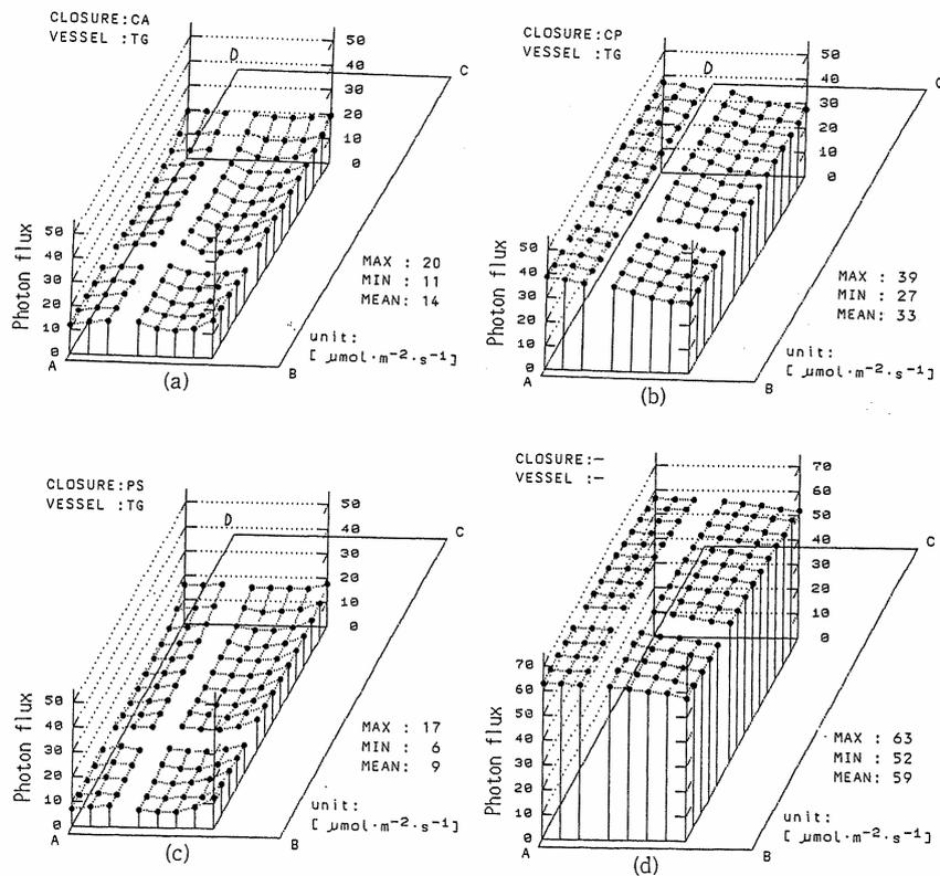
Figure 10. PPFs in the test tube type vessels as affected by types of vessel caps (Fujiwara et al., 1989). (a) aluminium foil caps, (b) polypropylene formed caps, (c) silicon rubber plugs, and (d) no caps. MAX, MIN and MEAN denote maximum, minimum and mean PPF, respectively.
