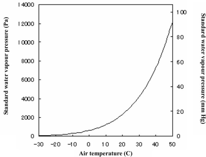
Figure 3. Saturation water vapor concentration or partial pressure as a function of air temperature.
