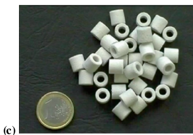
Figure 5. (a) A principle of catalyst 9 activation and non-covalent binding of a catalyst to polymeric phase; (b) Sulfonated polymer particles inside Raschig rings, as visualized by SEM; (c) Megaporous glass Raschig rings used for immobilization of 9 .
