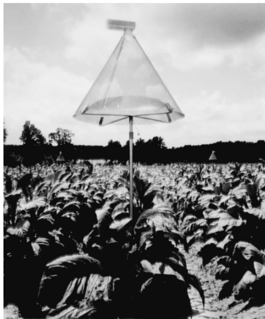
Figure 5. Photograph of plexiglass contamination station attached to a pheromone-baited wire-cone trap for autodissemination of nucleopolyhedroviruses
