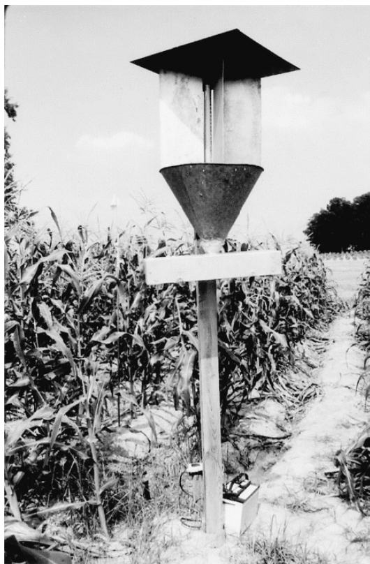
Figure 7. Photograph of aluminum contamination station attached to the bottom of a battery-powered blacklight trap for autodissemination of nucleopolyhedroviruses
