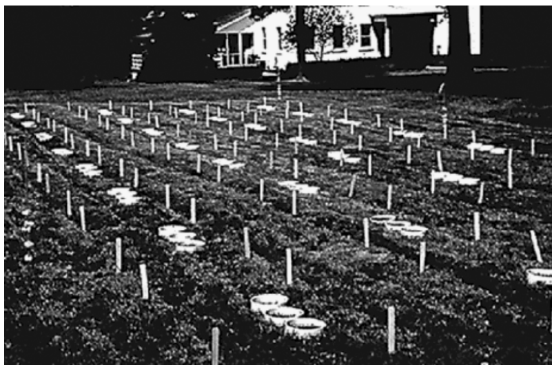
Figure 2. PVC cylinders in place for field test
